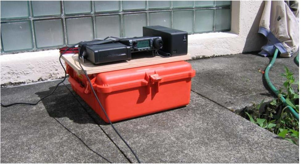
L-R Antenna Tuner, Radio and Power Supply with carrying case.
