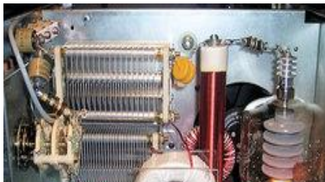
Eric Tichansky, NO3M, has modified a Heathkit SB-1000 linear for 630 meters, so he can generate sufficient power to obtain 1 W ERP.
