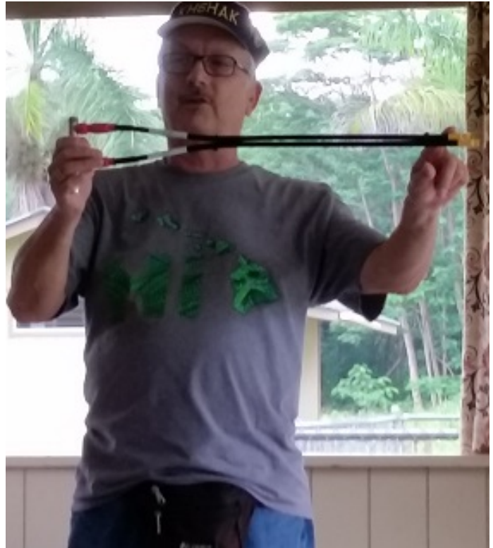
Two excellent 1/4 wave filters were built by Hank, KH6HAK, and presented to the club for installation at the Pepeekeo repeater site (146.28/88).
