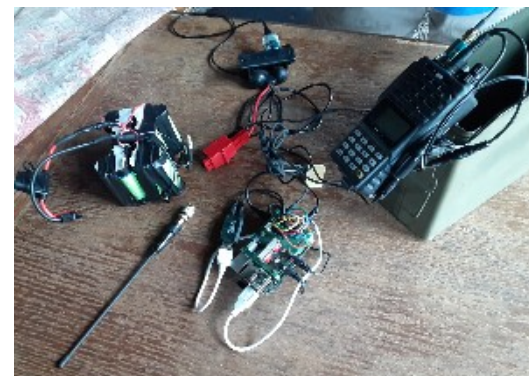
Inside the fox box: battery pack, radio, and raspberry pi to provide code message at 2-minute intervals.
