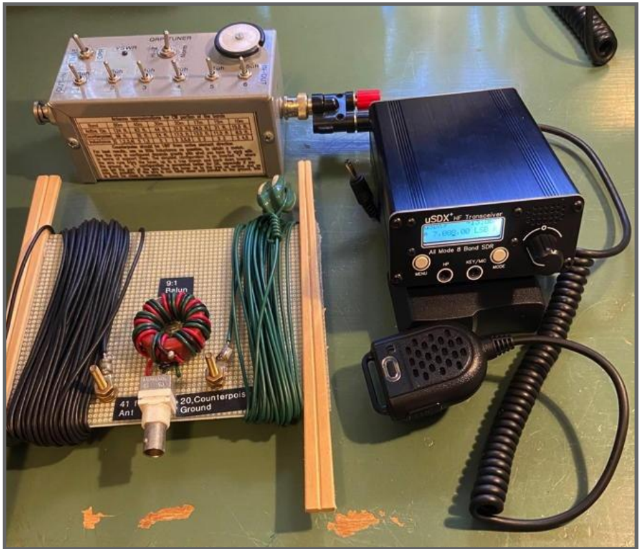
Meet the uSDX+ Plus, Version 2 QRPocket Transceiver. Little SDR unit plays well with FT8, Winlink, other digi modes.
